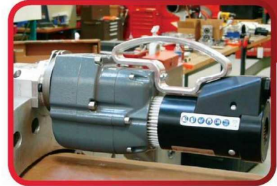
Once mounted, the lightweight EPM (Electric Power Motor) is out of the way.
