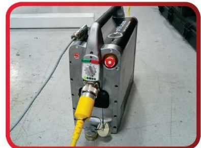
Power controller is compact and portable, includes lock out tag out closure and top mounted controls
