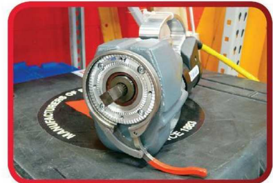
Standard drive insert works with LCSF Low Clearance Split Frame and EP 424 End Prep Machines
